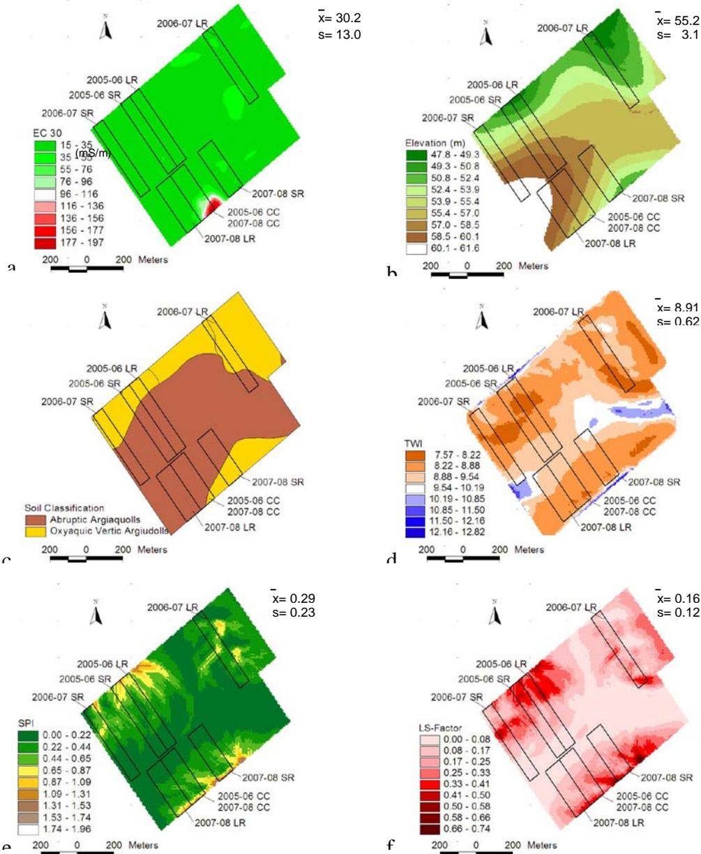
**Fig.2. Terrain attributes and soil classification at the experimental site for eight year\*rotation combination. (a) Electrical Conductivity at 30cm depth (EC 30), (b) Soil classification, (c) Elevation, (d) Topographic Wetness index (TWI), (e) Stream Power index (SPI), and (f) Length-Slope Factor (SL-Factor).**
